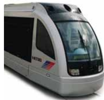
Siemens train window panel made with Ultem R16SG29 sheet. Use of Ultem R16SG29 sheet is growing in train window masks, cladding, walls and seating, and other interior parts
